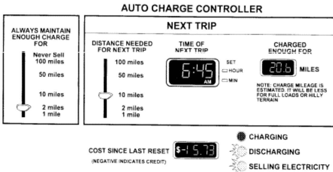
Figure 2.2. Suggested design of vehicle dashboard control, allowing driver to limit loss of range of vehicle and monitor power transactions (From Kempton and Letendre 1997). The control shown here is for a battery vehicle; similar controls would be used for fueled vehicles to limit the drawdown of the tank. These functions might alternatively be accessed via a web browser.
