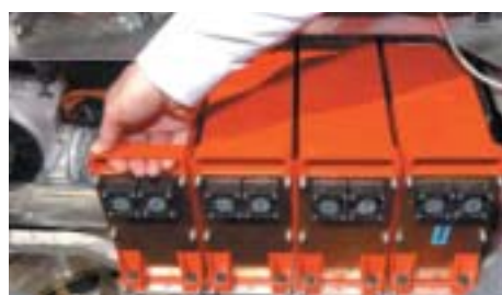
Exhibit 3.3 LA battery: spiral-wound cells – (a) individual 2 V cell; (b) complete battery module (source: ALABC/Energys)
