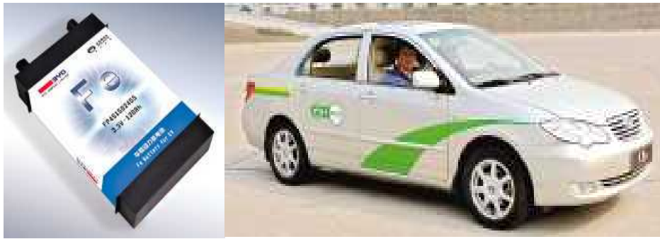
Figure 7 LiFePO 4 Battery of BYD and The E-car F3e
